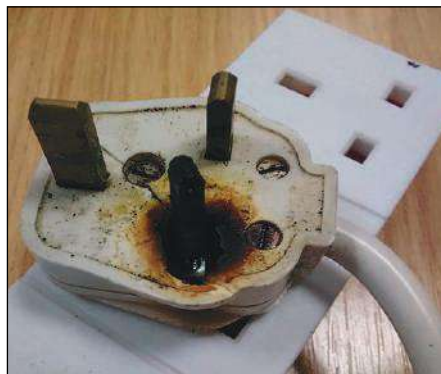
Plugs and chargers can be faulty and can easily go up in flames
